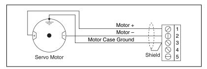
Figure 7. Typical Servo Motor (DC Brush Type) Terminal Block Pin Assignment
